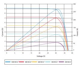
Excellent performance under weak light conditions: at an irradiation intensity of 200 W/m<sup>2</sup> (AM 1.5, 25 °C), **96.5%** or higher of the STC efficiency (1000 W/m<sup>2</sup>) is achieved
